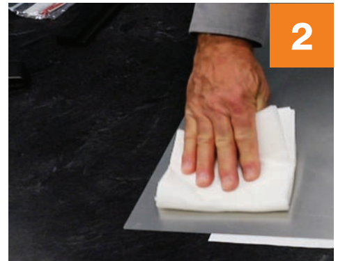
2 Clean the back of the ChromaLuxe® panel with isopropyl alcohol.
