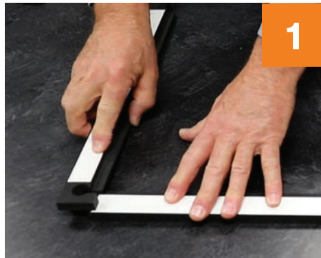
1 Assemble the frame by connecting the corners of the four frame sections.
